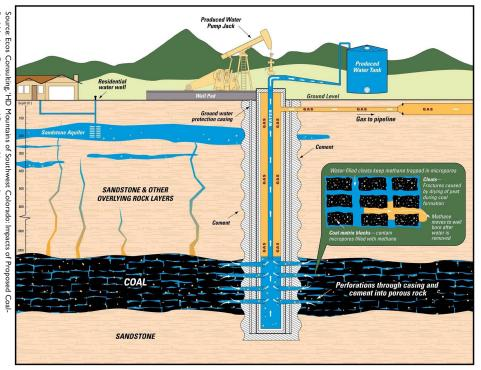
A cross section of a typical coalbed methane production well. In some regions the drinking water aquifer is located within the coal seam. Natural fissures located above the coalbed formation can provide possible conduits for contamination of underground sources of drinking water. During the hydraulic fracturing process the natural fissures can be expanded, facilitating further contamination.
