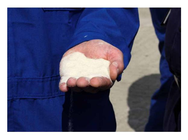
Photo 5.17 - Sand used in hydraulic fracturing operation in Bradford County, PA.
