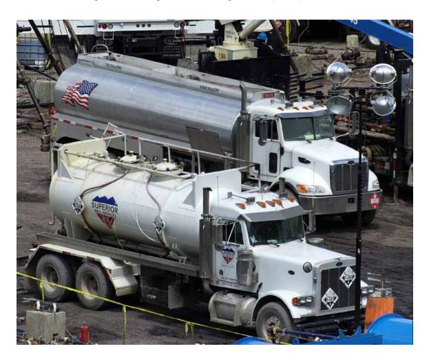
Photo 5.19 - Transport trucks for water (above) and hydraulic fracturing acid (HCl) (below)
