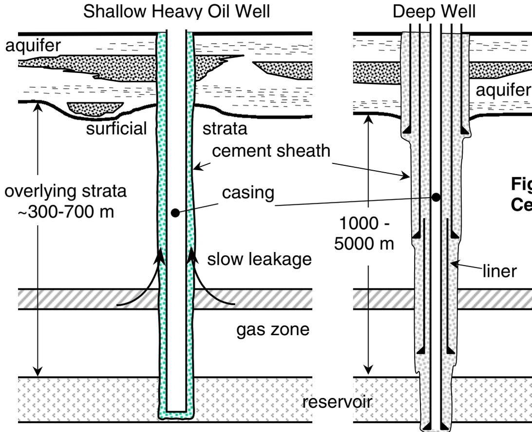
**Figure 1: Cased, Cemented Wells**
