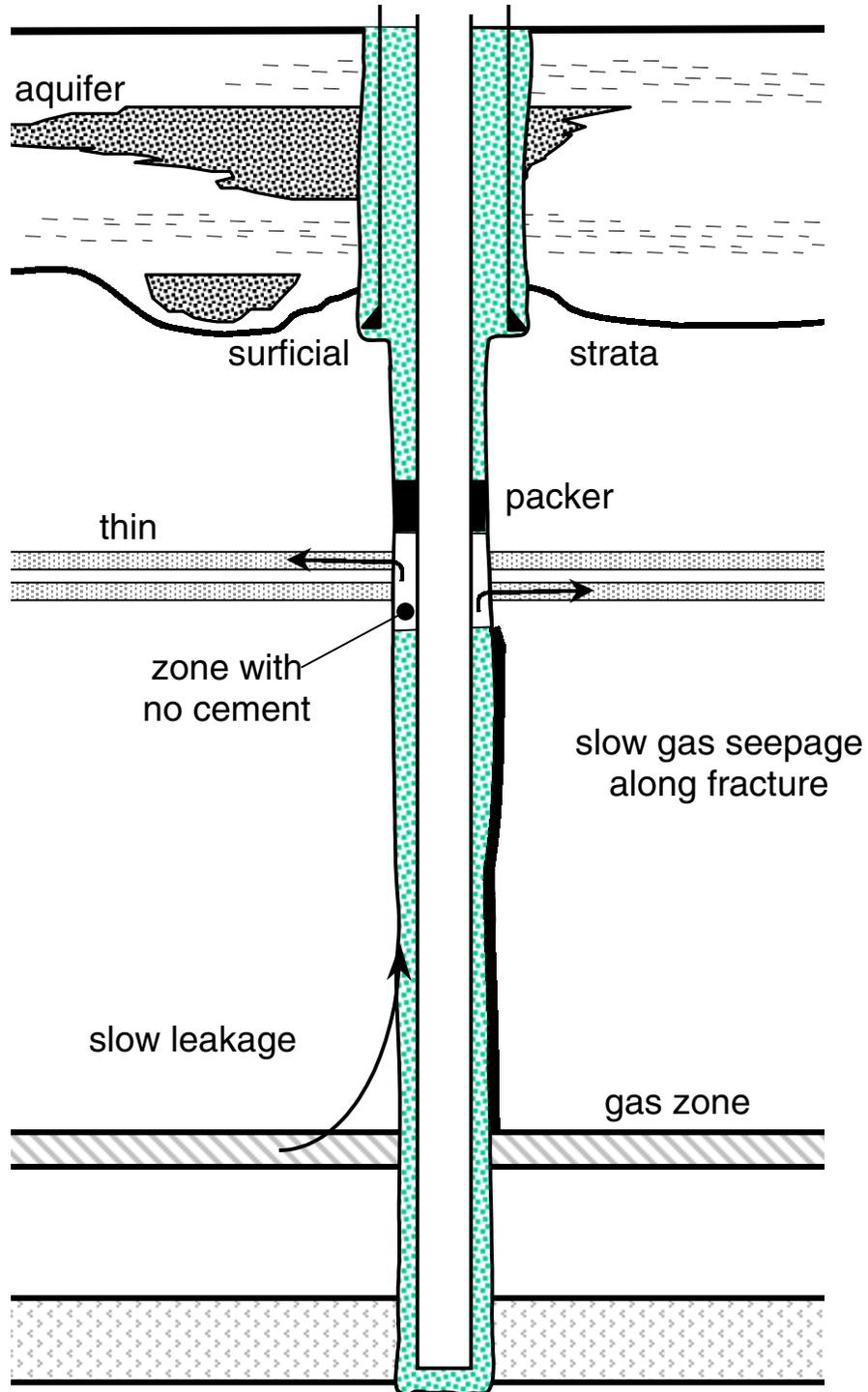
**Figure 5: Leaving a Leak Off Zone to Arrest Gas Seepage**
