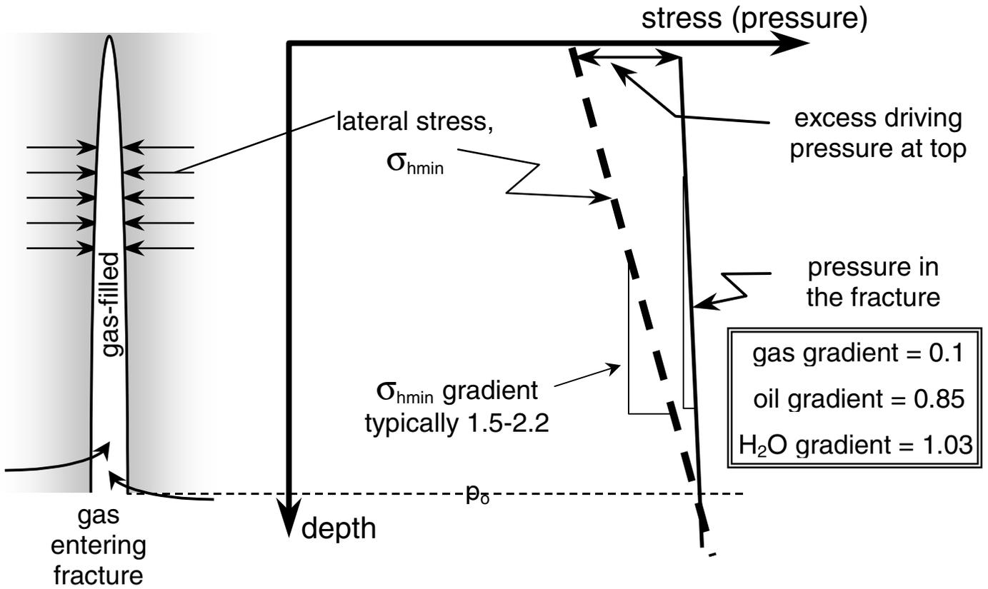
**Figure 3: Fracture Driving Pressure from Gradient Differences**
